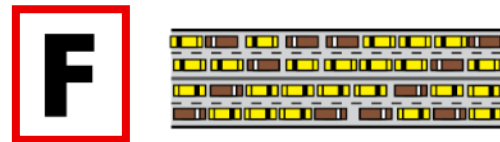
F Forced flow with demand volumes greater than capacity resulting in congestion.
